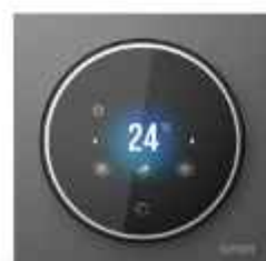
82E701 ★ S20 Central AC thermostat Module (DC12V, RS485, Modbus open protocol, available for third party RCU system VRF)
